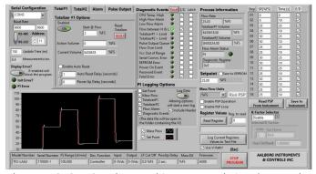
The AALBORG TIO LabVIEW drivers were designed to make communication with TIO instruments using LabVIEW much easier, and include drivers will work on any TIO instrument that is configured for RS-232 or RS-485 interface and store historical data.
