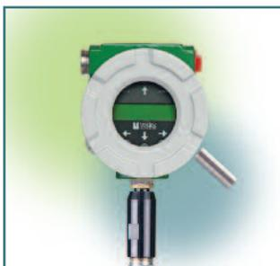
VorTek Instruments' Pro-V™ multivariable flowmeters utilize three primary sensing elements—a vortex shedding velocity sensor, an RTD temperature sensor, and a solid-state pressure transducer—to measure the mass flow rate of gases, liquids and steam. Because the Pro-V™ is able to measure all process variables within a single device it provides exceptional accuracy, simplifies system design and reduces installation costs.
