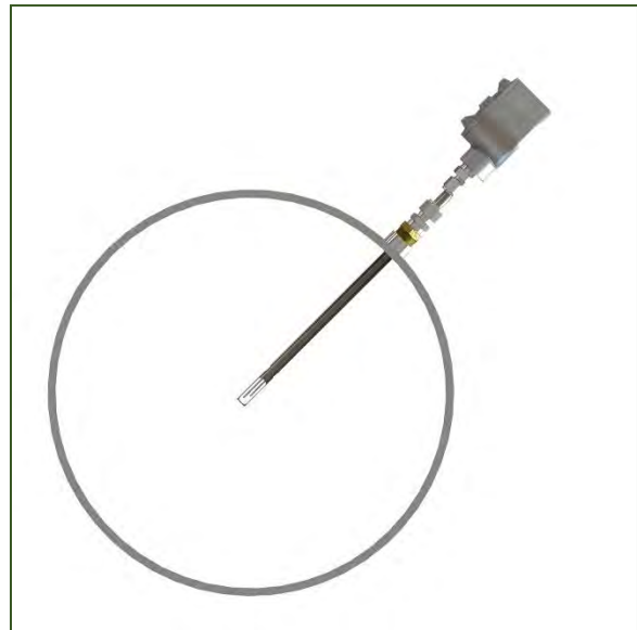
Angling the flow sensor in the pipe can help combat inaccuracy associated with condensed moisture.
