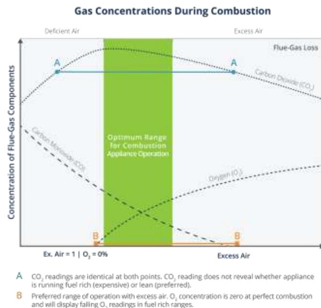
Figure 7: O<sub>2</sub> vs CO<sub>2</sub> Measurements in Combustion Analysis
