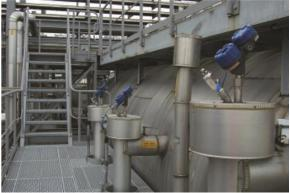
Pipeline specifications require removal of CO2 and H2S. H2S is highly toxic and corrosive to carbon steel. CO2 is corrosive and reduces BTU value. Gas sweetening processes remove these
