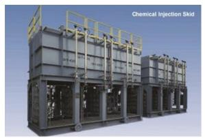
Chemical agents are frequently administered by chemical injection skids. Chemicals employed in natural gas processing include drilling fluid additives, methanol injection for freeze protection, glycol injection for hydrate inhibition, produced water treatment chemicals,
