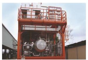
Natural Gas Dehydration removes hydrates which can grow crystals and plug lines and slow down flow of gaseous hydrocarbon streams. Dehydration also reduces corrosion, eliminates foaming, and prevents problems with catalysts downstream. Compressor stations often use a liquid separator to dehydrate natural gas prior to compression.
