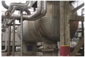
Liquid in the vent stream can extinguish the flame or cause irregular combustion or smoking. Flaring liquids can generate
