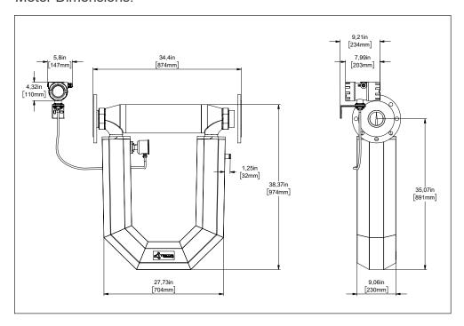
weight: 87 kg/194.4 lb with junction box & remote field mount meter connection: depending on selected connection
