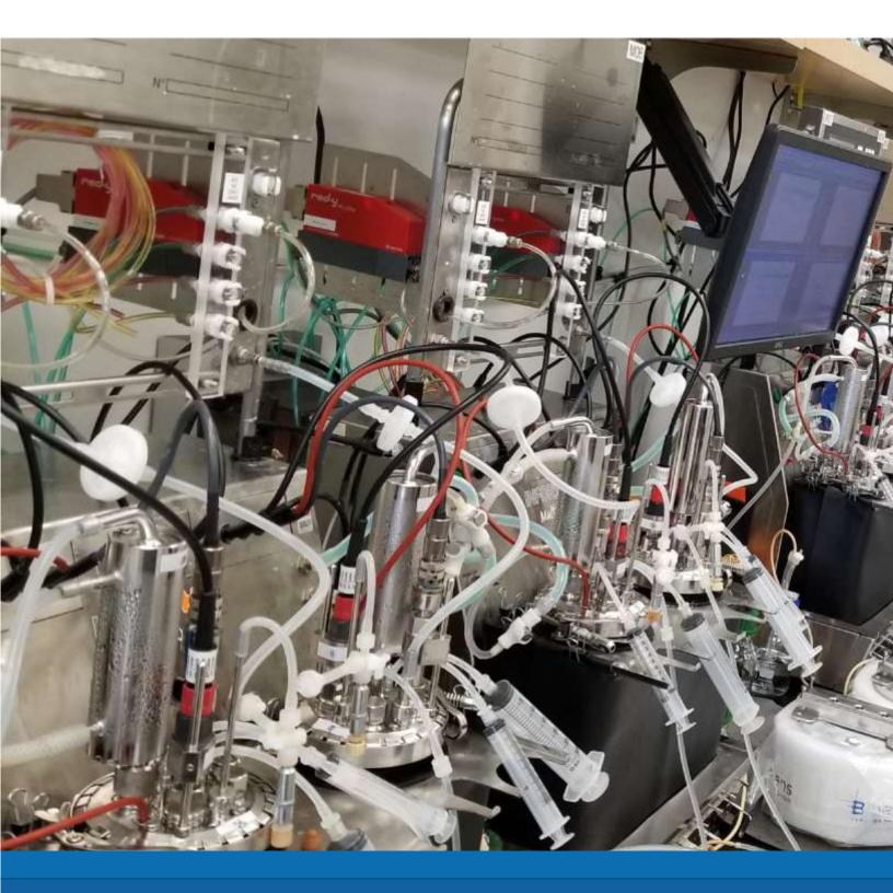
**APPLICATION SPOTLIGHT** Mass Flow Controllers Ensure Accurate Bioreactor Process
